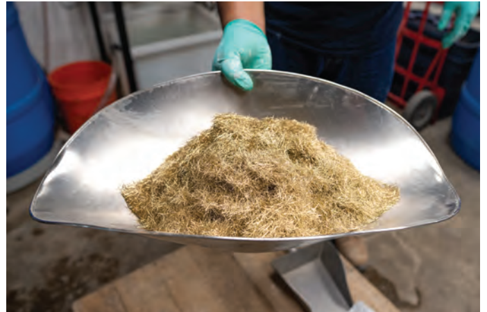
Typical steel fibers used in UHPC (photo courtesy of CTLGroup)
