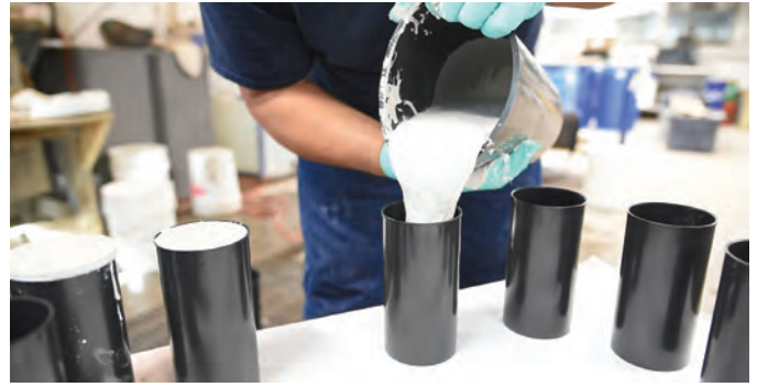
UHPC cylinder sample fabrication. UHPC contains properties similar to self-consolidating concrete (SCC) (photo courtesy of CTLGroup)
