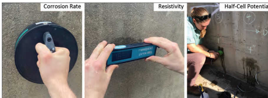
Fig. 6: Nondestructive techniques implemented.
