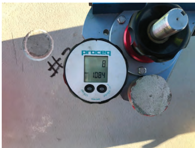
Fig. 7: Bond testing equipment (note specimen pull-off within overlay concrete matrix (photo courtesy of SK&A))
