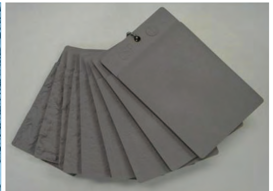
Fig. 3: ICRI CSP comparator chips
