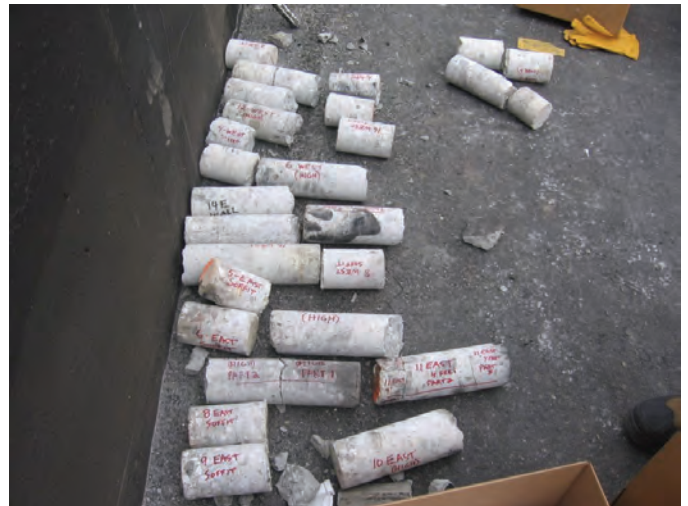
Fig. 5: 103 concrete samples were extracted from the undercrossing and examined in WJE laboratories in Illinois, Texas, and Ohio. Photo source: Wiss, Janney, Elstner Associates, Inc.
