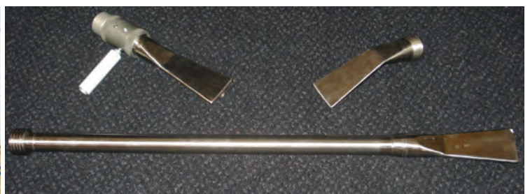
Fig. 6: Various blast nozzles
