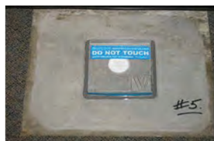
Fig. 3: Using an Anhydrous Calcium Chloride test
