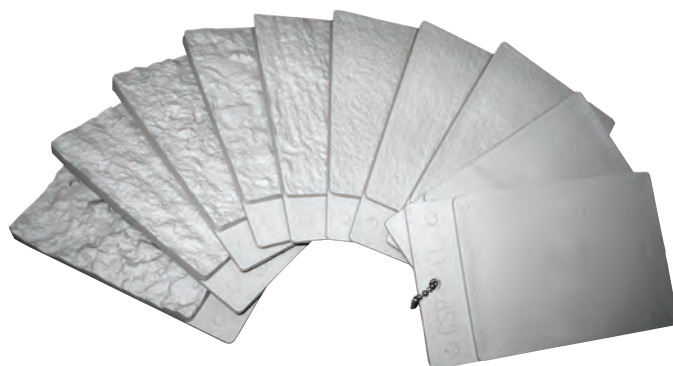
Fig. 5: ICRITechnical Guidelines, Surface Profile Chip Set
