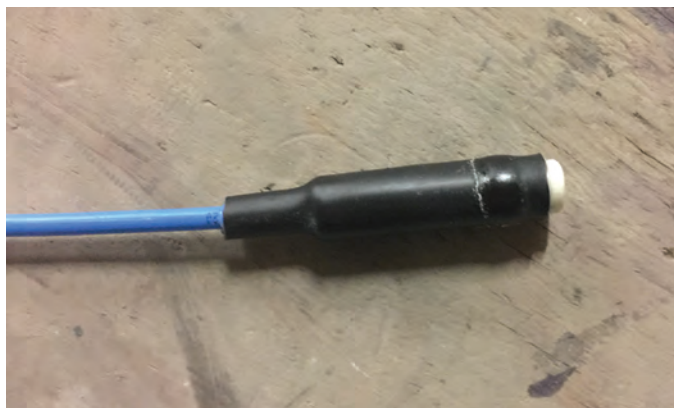
Fig. 6: The reference electrode is one of various types of sensors used to measure corrosion activity in concrete—newer sensors are smaller, reliable, and cost effective
