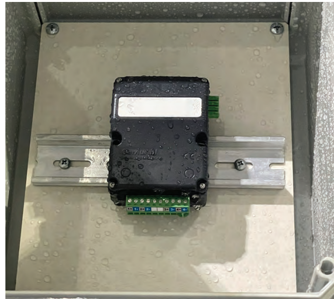
Fig. 8: Analogue to digital converter capable of monitoring four corrosion sensors—this technology allows digitization and management of large amounts of data efficiently as designs are “plug and play” and can be easily scaled or modified to accommodate cathodic protection systems if needed (Photograph courtesy of No Corrosion, LLC, West Palm Beach, Florida)
