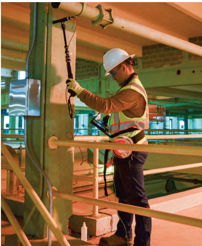
Fig. 5: Inspector performing half-cell potential testing
