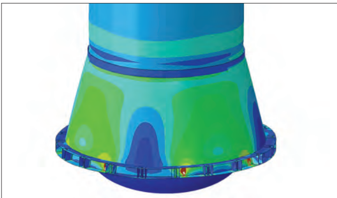
Fig. 9: Image from detailed finite element model used to assess catalytic reformer vessel and skirt during concrete removal
