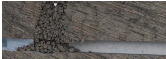
Fig. 2: Schematic illustrating internal collapse of the GAD tunnel as a result of growing pressure within the soil 7
