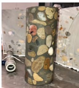
Fig. 8: Core taken from the proof of concept demonstration exhibits excellent consolidation
