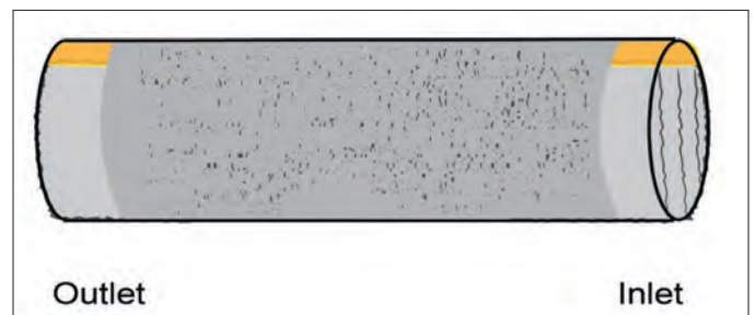
Fig. 6: Once the pre-stoppers are constructed, the debris within the tunnel can be excavated and a permanent concrete backfill can be installed
