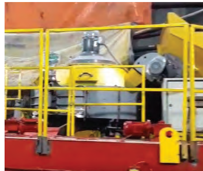
Fig. 14: Large mixer used to mix 1545 lb (700 kg) batches
