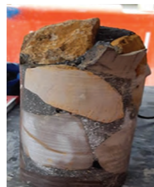
Fig. 12: The core taken from the field trial demonstrated excellent consolidation
