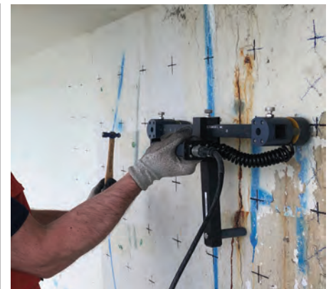
Fig. 9: Spectral analysis of surface waves method (SASW) and SASW bar with 2 receivers testing across surface-opening crack on girder
