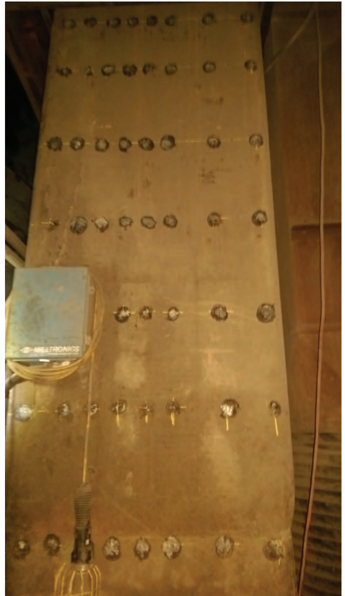
Fig. 2: Column layout for pulse velocity testing
