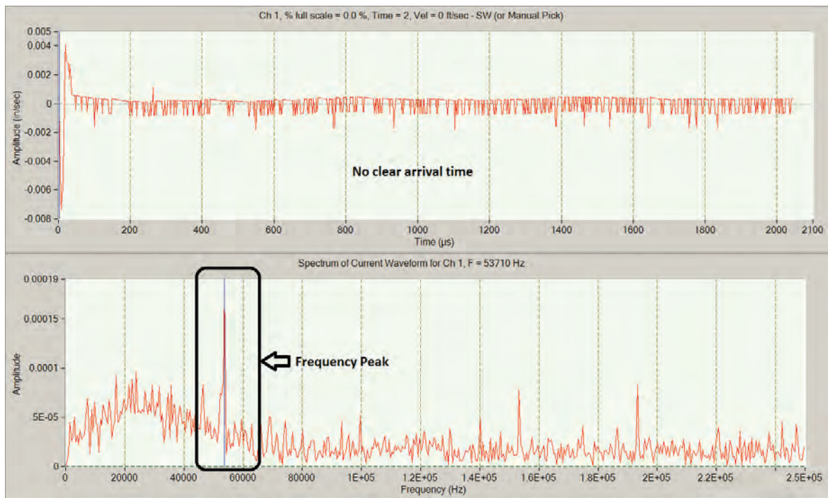
Fig. 4: Poor signal through concrete
