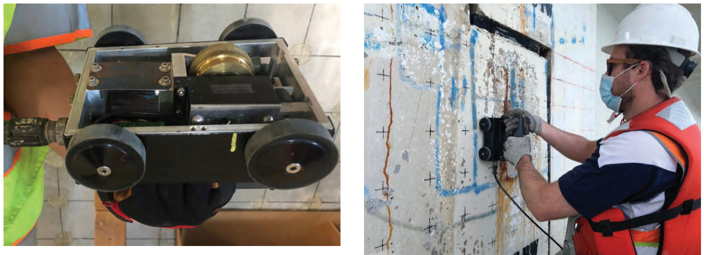
Fig. 7: Impact echo scanner with rolling transducer wheel and solenoid impactors (left) and impact echo scanning of girders on vertical lines at 6 in (150 mm) spacing (right)
