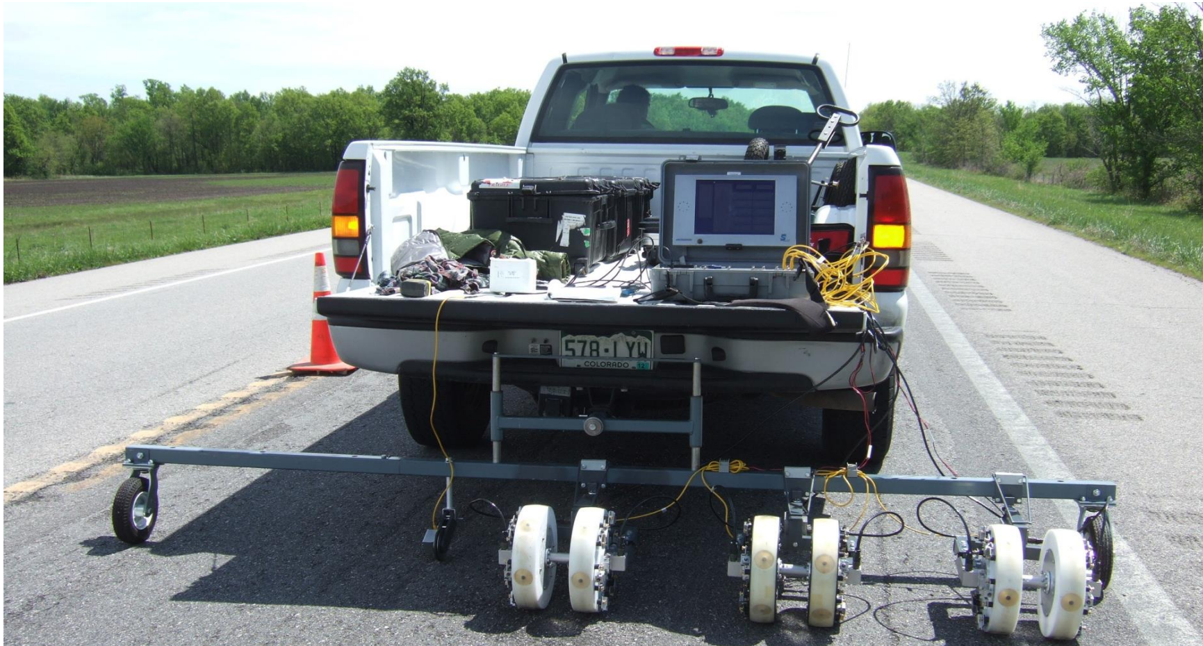
Pavement Scanner on Kansas Asphalt Pavement site with 3 pairs of wheels spaced 150 mm (0.5 ft) apart for combined Impact Echo and Spectral Analysis of Surface Waves scanning.
