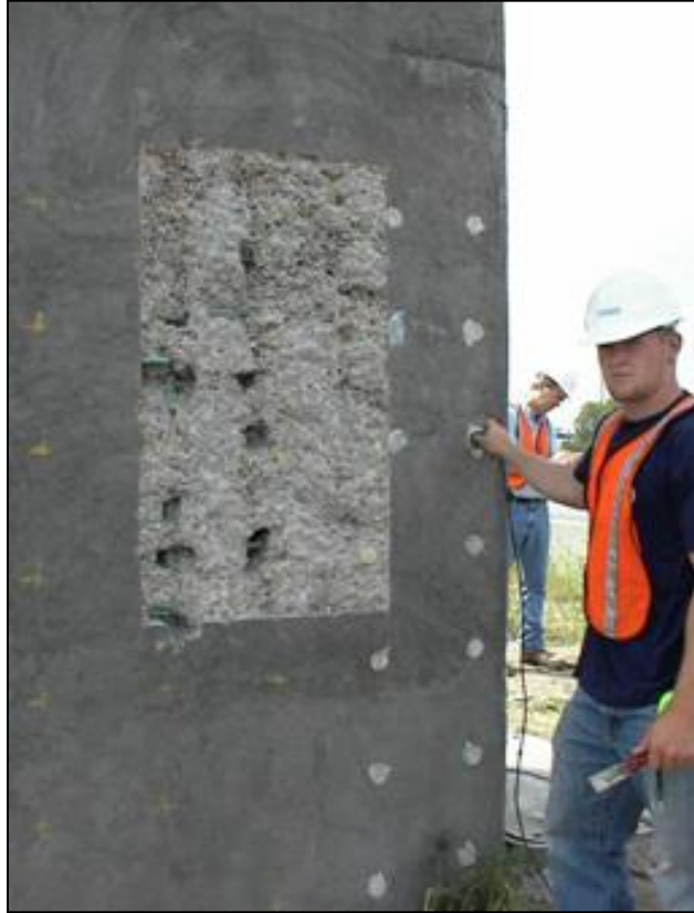
54 kHz UPV transducers with 1 ft grid direct test patterns from North-South and East-West
