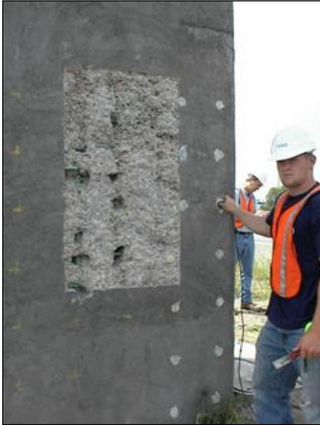
54 kHz UPV transducers with 1 ft grid direct test patterns from North-South and East-West
