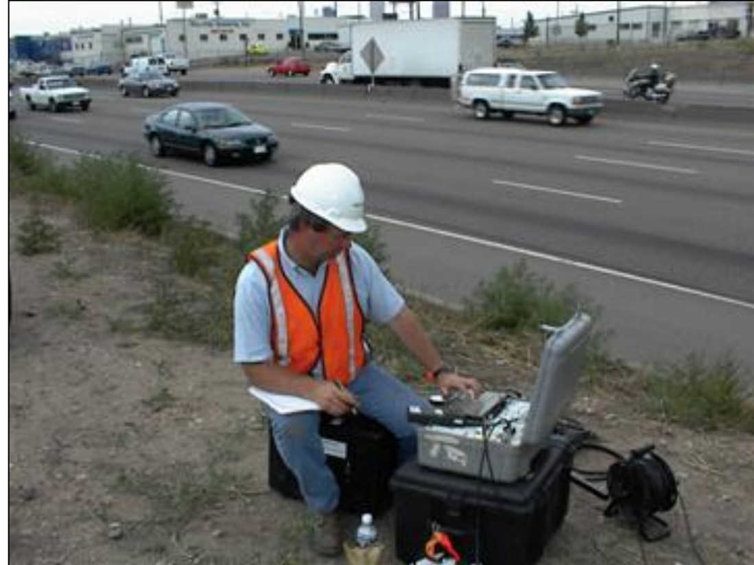
UPV test data recorded for pulse velocity arrival time analyses on Freedom NDT PC
