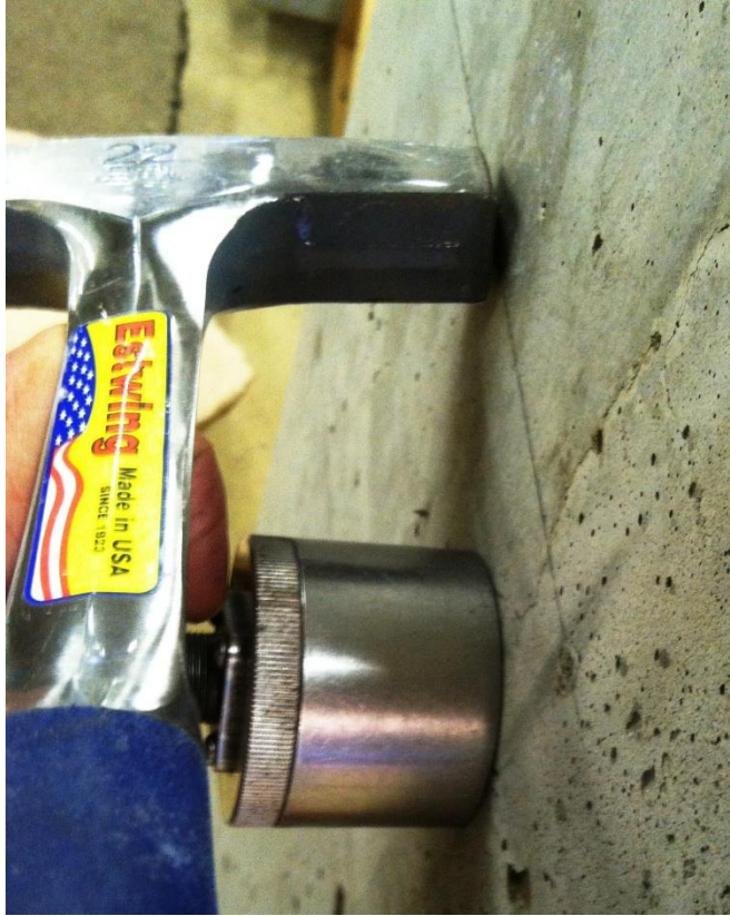
Hammer Source with UPV Transducer Trigger
