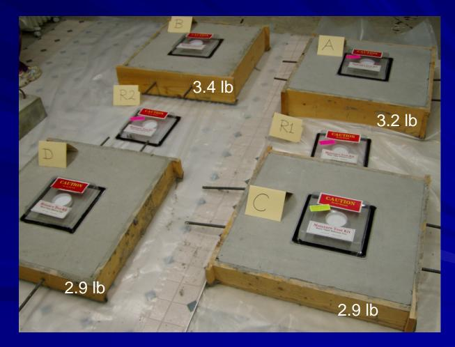
Mix Design: 4,000 psi, **w/c = 0.4**, 7-sack mix, **15%** Fly ash, slump =3-4"
