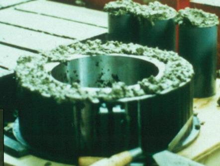
Criteria No cracking <14 days age 0.10% max implied strain
