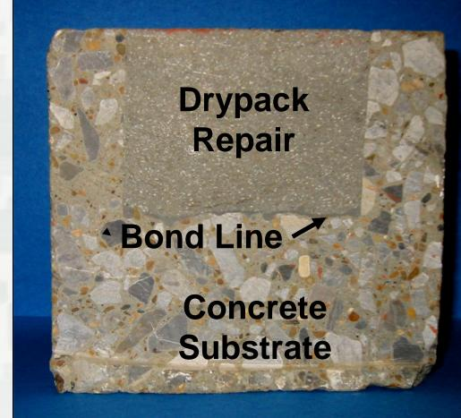
A repair produced by combining different materials (e.g., concrete substrate, bonding agent, and repair material) which are so interconnected that the combined components act together as a single unit.
