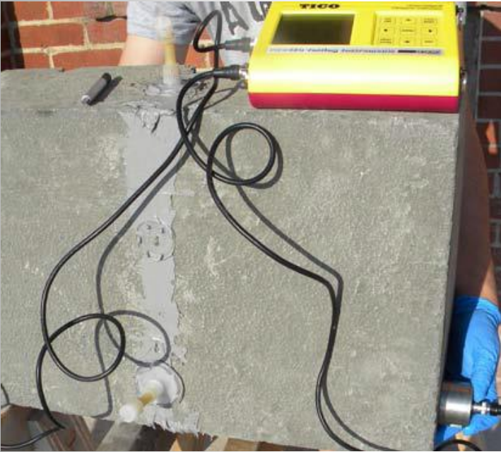
Ultrasonic Pulse Velocity measurement on fractured concrete slab
