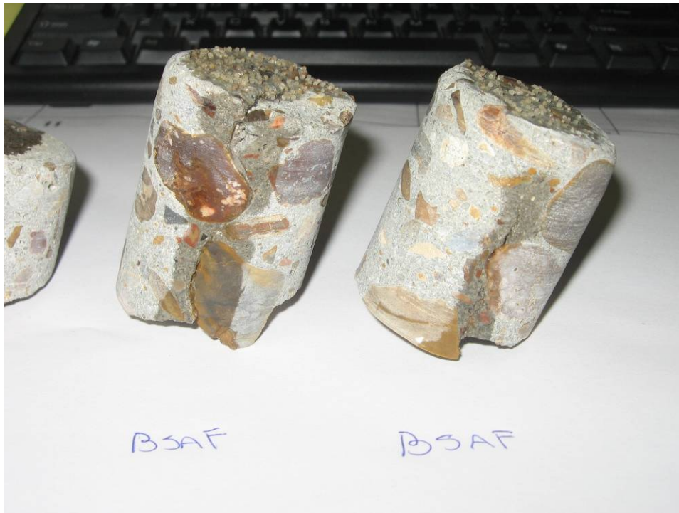
MMA Crack Sealer cores
