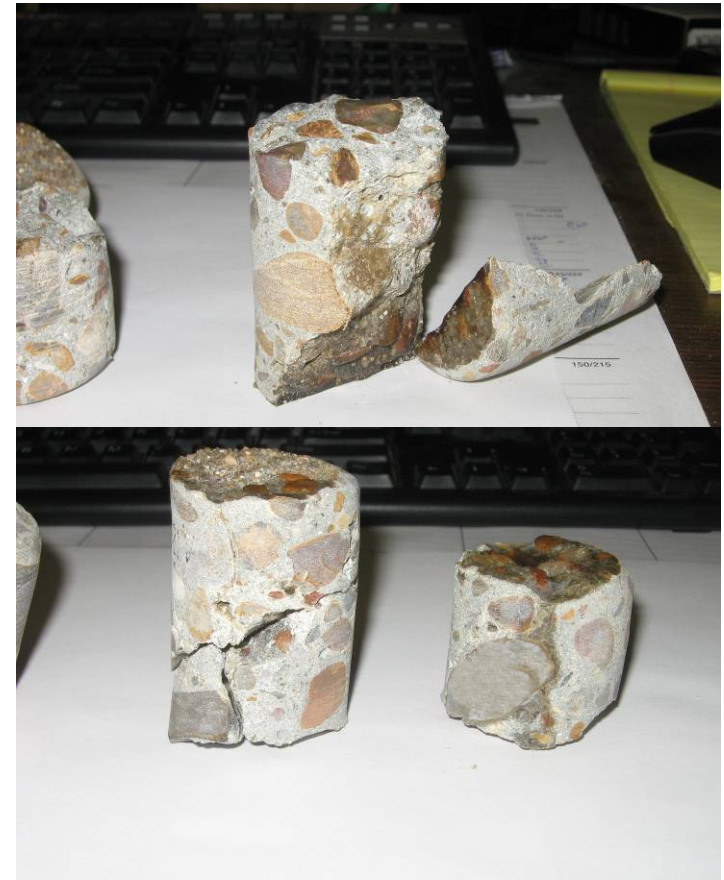
Epoxy resin cores: Lesser penetration and adhesion
