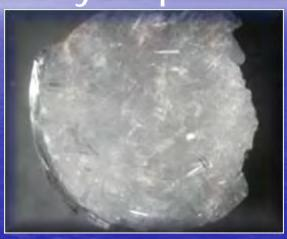
Fig. A-B: Shows the 2 types of crystals. The crystals form inside the pores, capillaries and voids to stop and block moisture when present. When moisture is no longer present the hydrophilic crystal shrinks to allow the concrete to breath naturally.
