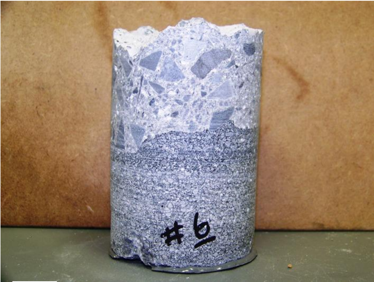
Overall of bond test core with failure within the substrate concrete.
