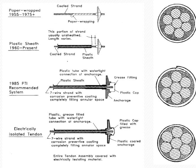
Fig. 3.2—Evolution of corrosion protection for unbonded single strand tendons for buildings (reprinted from Reference 2).
