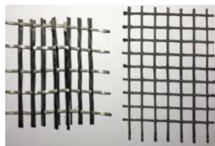
Figure 2. FRCM unidirectional (left), bidirectional (right).
