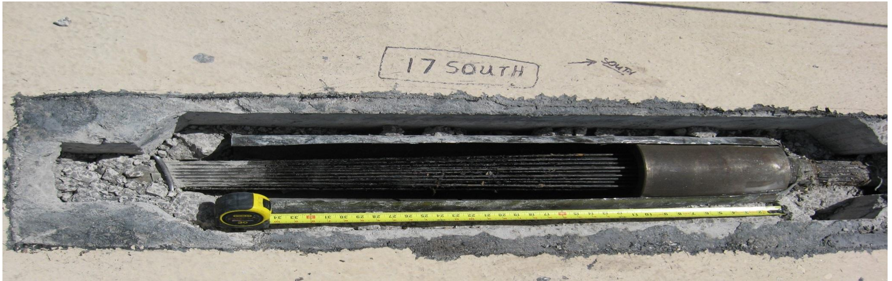
Photo #3 (above) shows cable coupling in normal position, with straight parallel wires. This occurred at the un-failed end.
