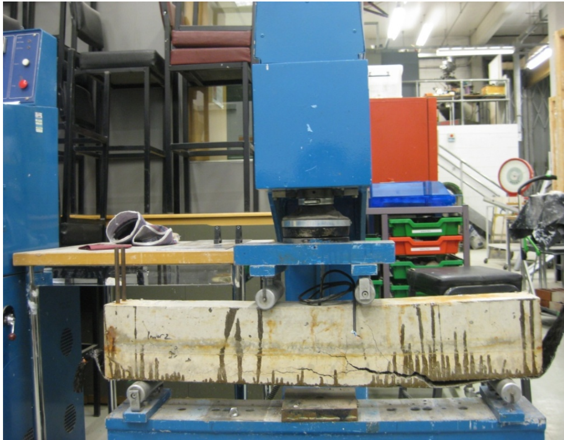
Bending test of dual functional CFRP fabric beams at ultimate load
