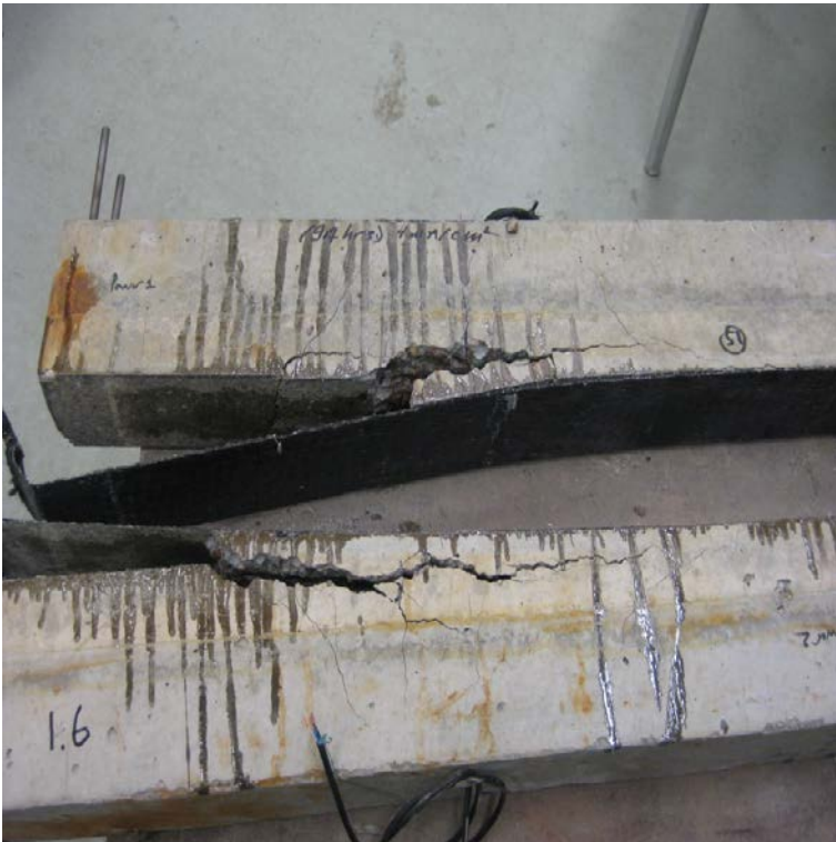
CFRP fabrics - after testing Failure in concrete
