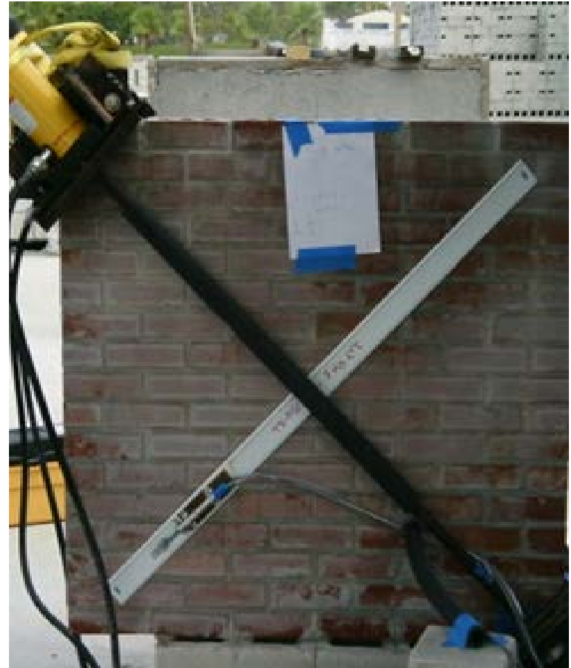
Clay brick-control wall
