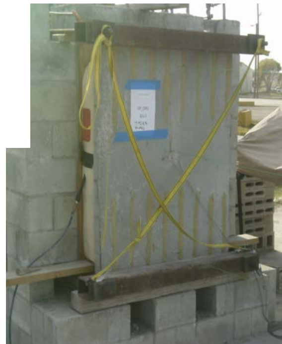
CMU wall with 4-ply FRCM
