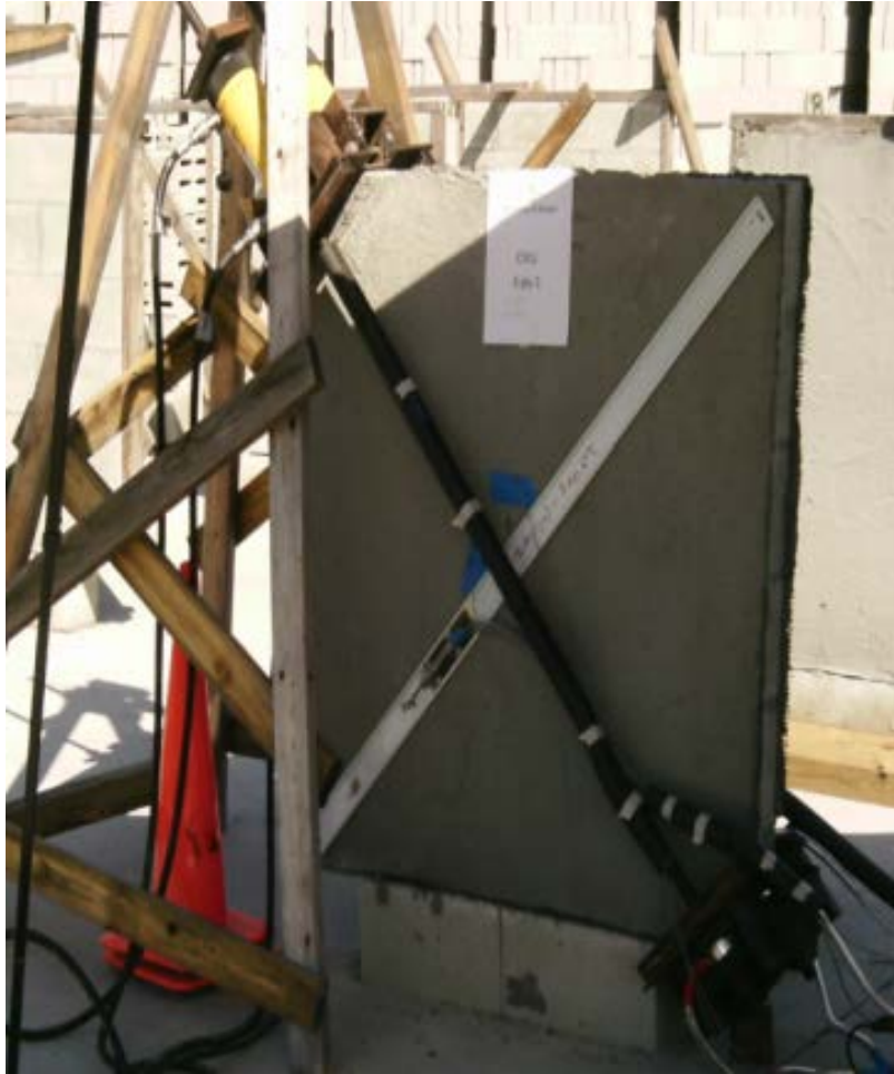
CMU wall with 1 ply FRCM
