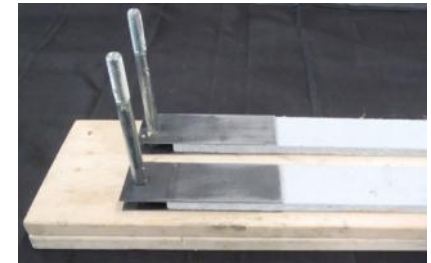
Align and glue metal tabs
