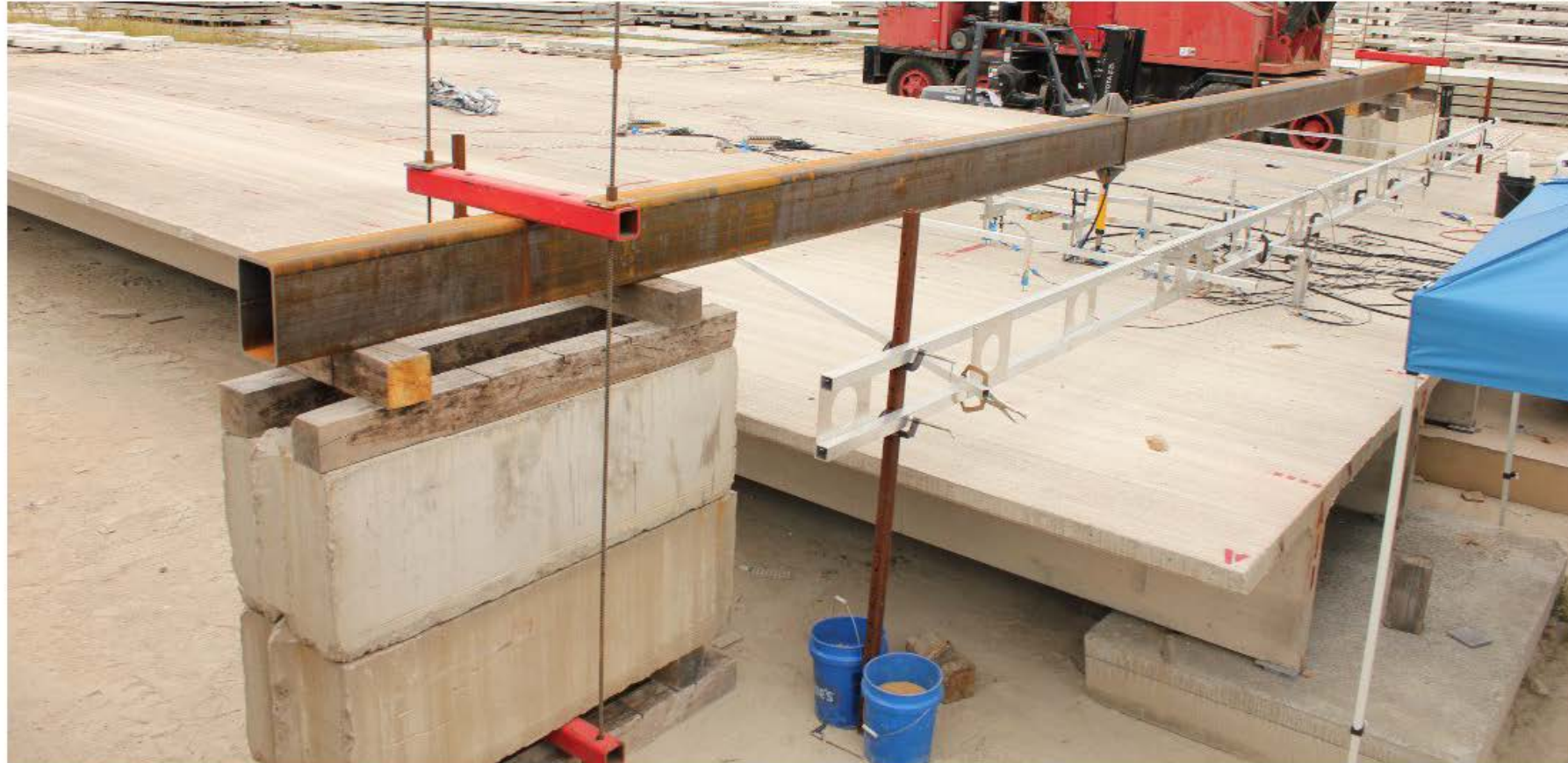
Figure 11: Test Setup with Loading and Instrumentation Frames 7.5 ft from End of Double Tees
