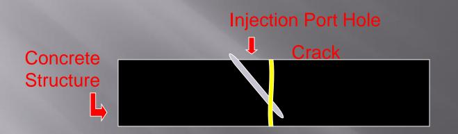
To drill at a 45° angle drill distance must be ½ the thickness of the wall.
