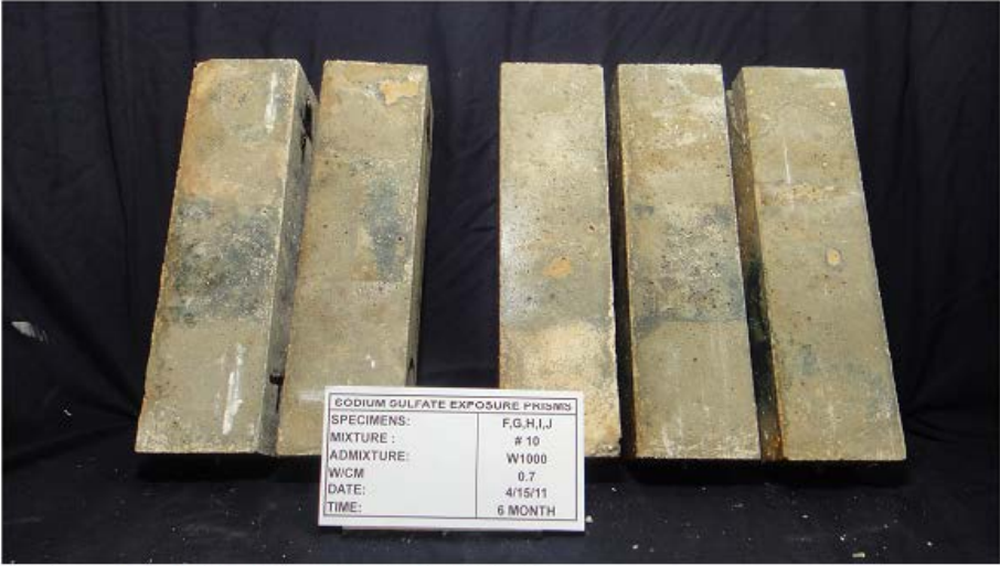
Figure 4: Mixture 10 Set 2 Prisms after 6 months of Exposure
