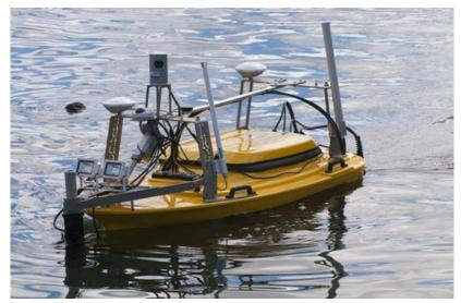
Rapidly deployed Unmanned Surface Vehicle (USV) that assesses pilesupported marine structures.
