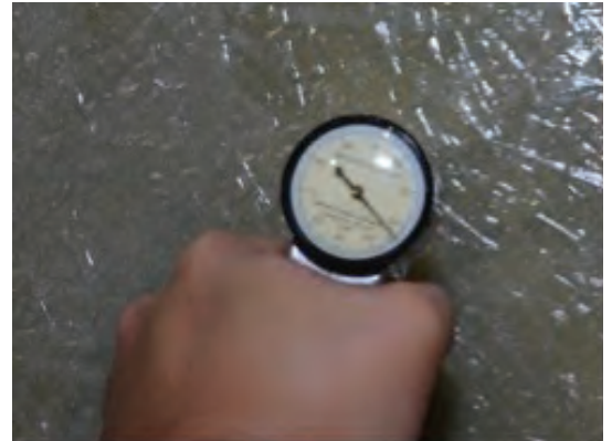
Fig. 4: Barcol hardness test for resin cure
