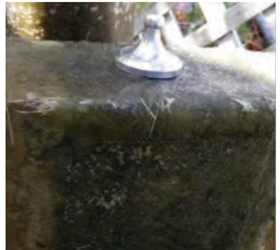
Fig. 5: 2.0 in (50mm) test dolly adhered to a prepared FRP laminate
