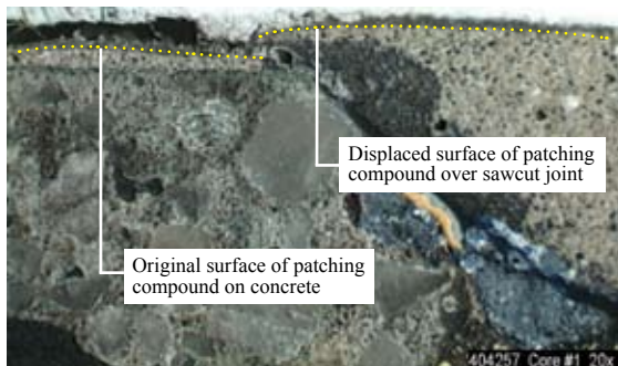
Fig. 4: Photomicrograph in reflected light showing details of patching compound movement upward. Dotted lines indicate original surface and displaced surface due to movement. The black gap at top left is the space created when tile was pulled loose from the patching compound, forming a bubble
