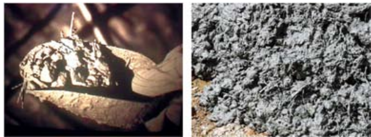
Fiber-reinforced concrete promotes better control of crack formation and propagation
