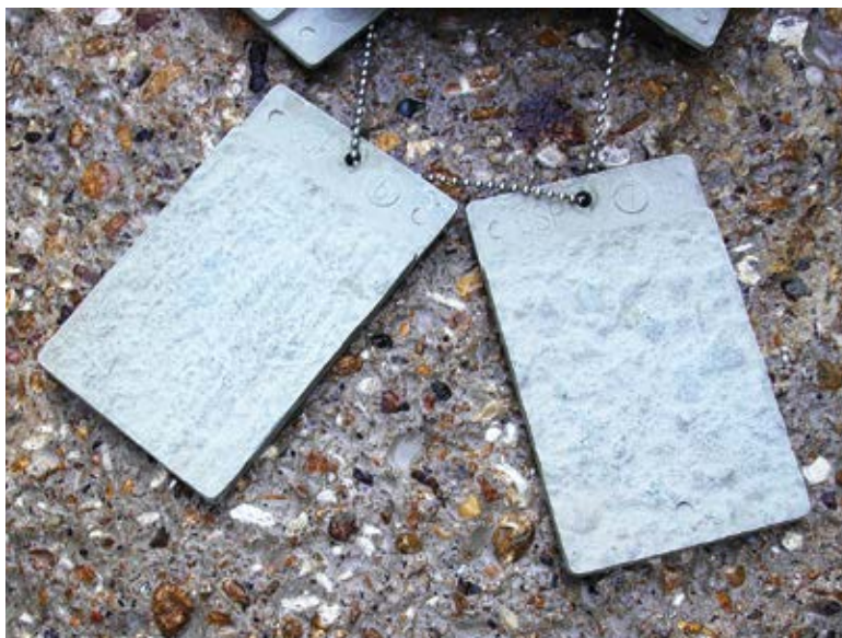
Fig. 3: Concrete surface profile (CSP) chips on prepared surface
