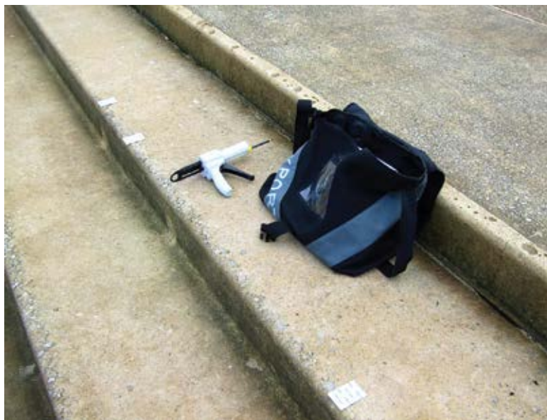
Fig. 8: Surface that was copied using silicone-based replicating polymers
