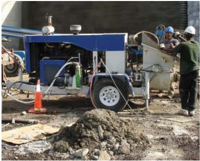
Fig. 4: Wet-mix shotcrete pump
