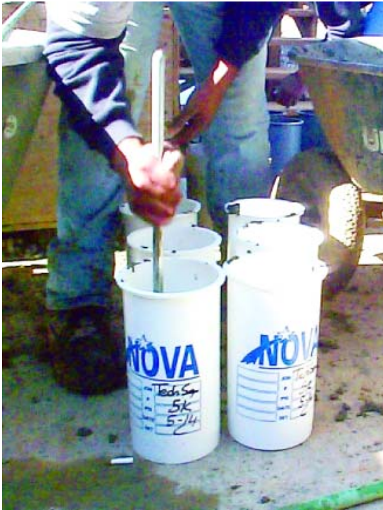
Figure 4: Rodding the cylinders in the mold
