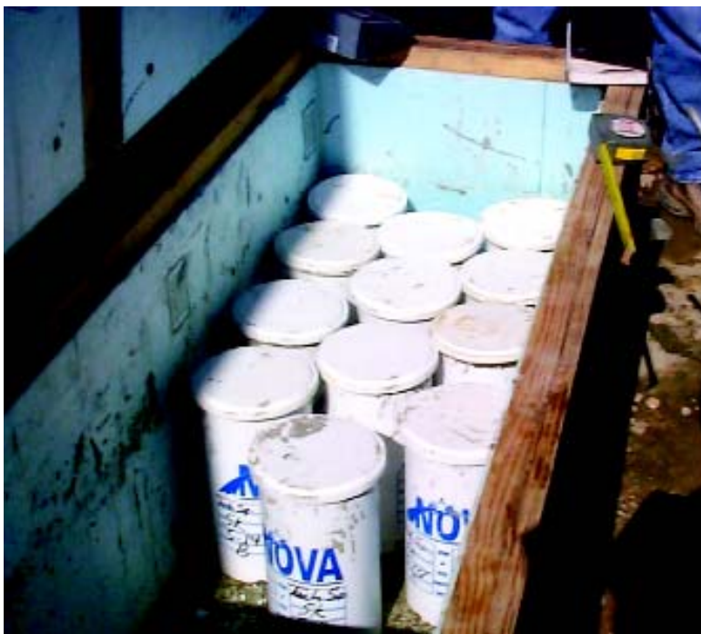
Figure 5 and 6: Cylinders in an insulated storage box
