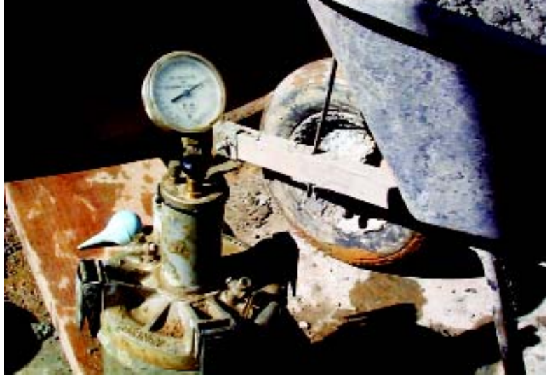
Figure 1: Testing for air content using a pressure meter
