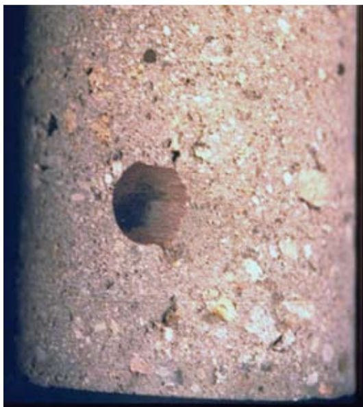
Fig. 3: Low permeability “labcrete”
