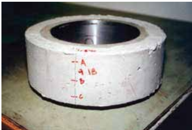
Fig. 3: Typical ring test specimen
