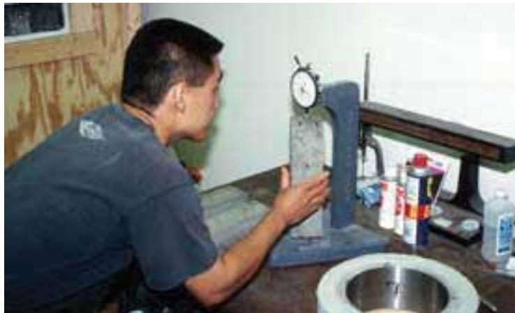
Fig. 1: Typical comparator for length-change measurements
