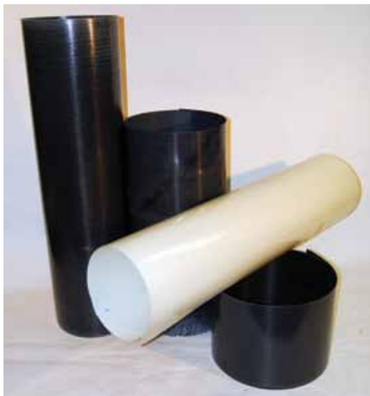
Fig. 2: Sample rolls of FRP laminates
