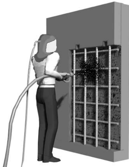
Cleaning of reinforcing steel and concrete with abrasive blast.
