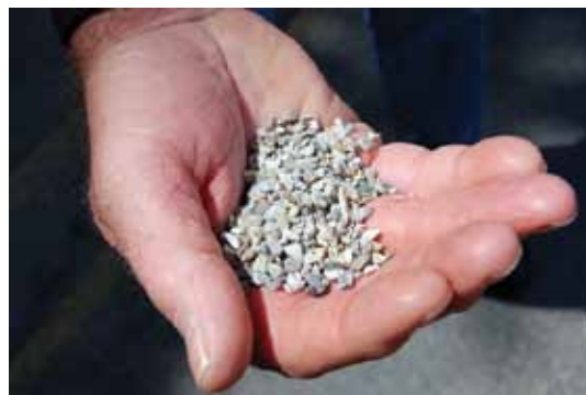
Fig. 1: Flint rock aggregate broadcast into epoxy for nonslip surface
