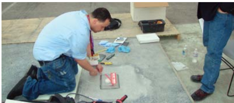
Applicant performing ASTM F1869
