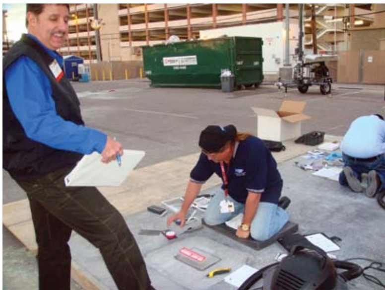
Judge Lee Eliseian tests one of the applicants on their knowledge of ASTM F1869
