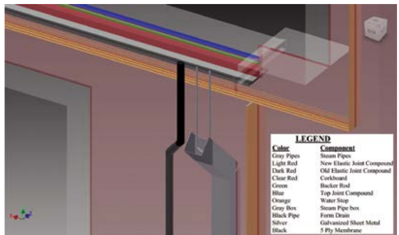
Fig. 5: 3-D drawing of expansion joint at Folsom Dam
