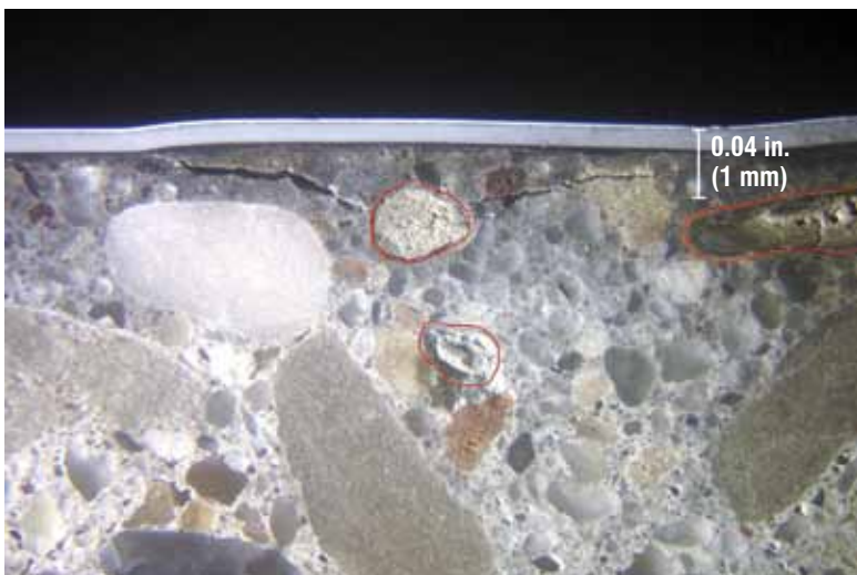
Fig. 7: ASR shale fine aggregate particles have formed protrusions in the coating system
