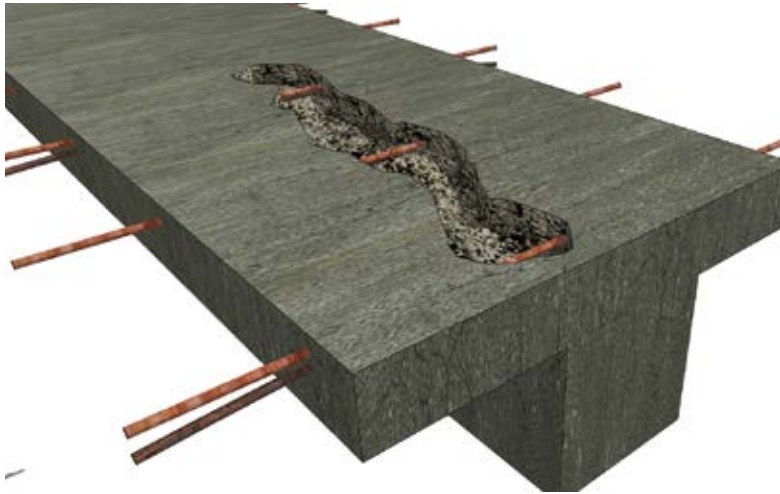
Fig. 3: Schematic view of concrete spalls in a PT slab
