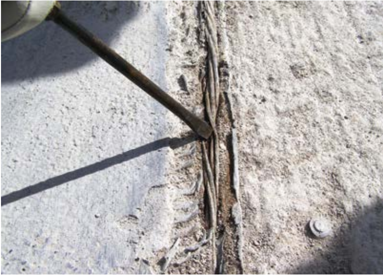
Fig. 5: Overview of screwdriver penetration test
