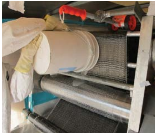
Fig. 7: Saturation of carbon-fiber fabric
