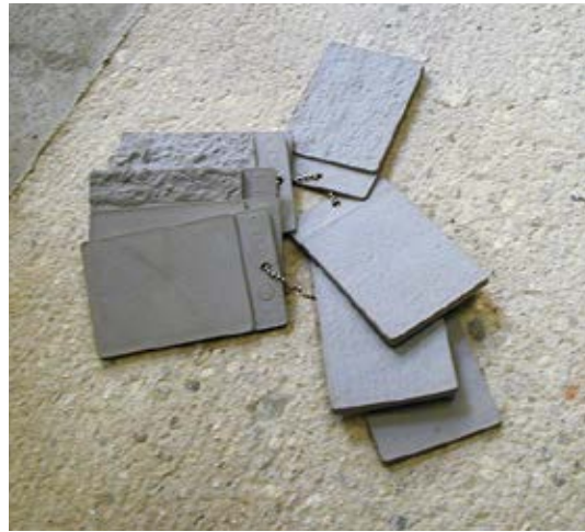
Fig. 6: CSP chips on prepared surface
