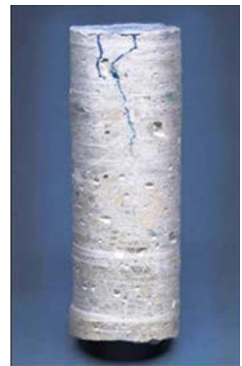
Fig 4: Epoxy healer-sealer penetration into concrete cracks as large as 0.002 in. (0.05 mm) Photo courtesy of Dayton
