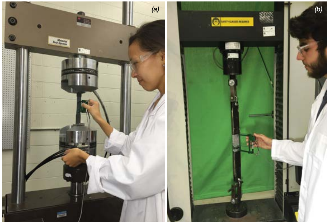
Fig. 1: Tensile tests of (a) FRP; and (b) FRCM coupon, according to AC125 and AC434
