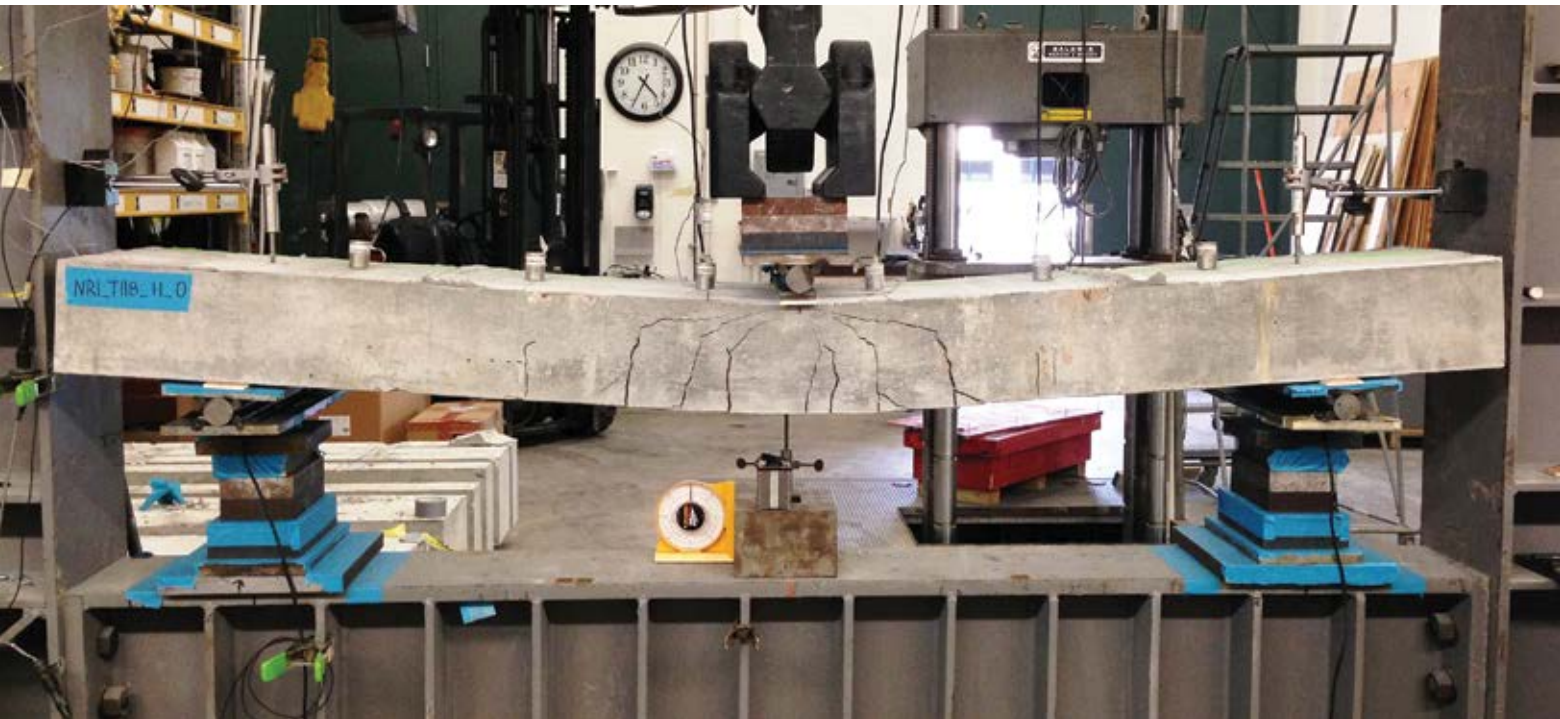
Fig. 3: Flexural test of RC slab strengthened with FRP for design validation, according to AC125
