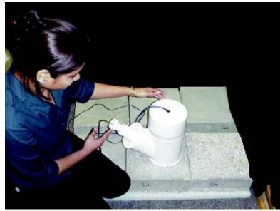
Figure 5: Prototype of the laser profiling device, measuring six manufactured concrete surface profiles
