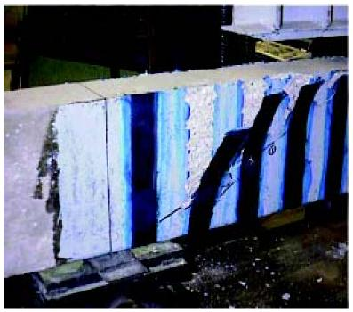
Figure 2: Delamination of externally bonded FRP sheets
