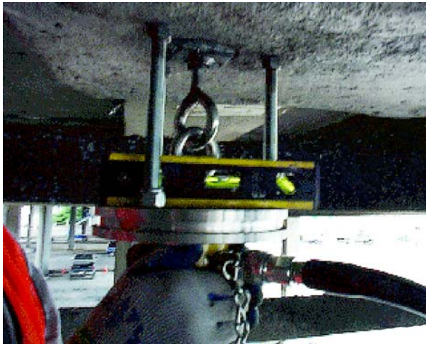
Figure 1: Tensile bond test setup
