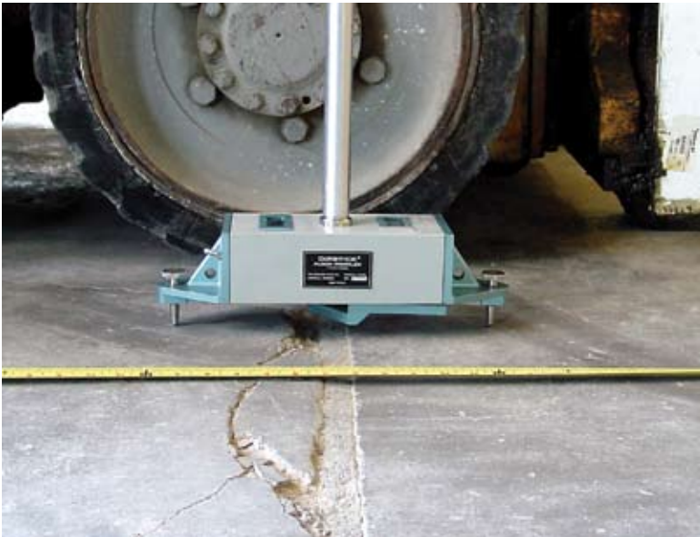
Fig. 6: A dipstick floor profiler being used to measure joint stability
