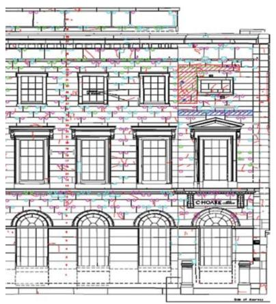
Fig. 6: CAD representation of iron component positions including color-coding of corrosion risk assessment. Note that the red-shaded area was the location chosen for the ICCP preview study. The blue-shaded area was to test surface-applied corrosion inhibitors that did not take place
