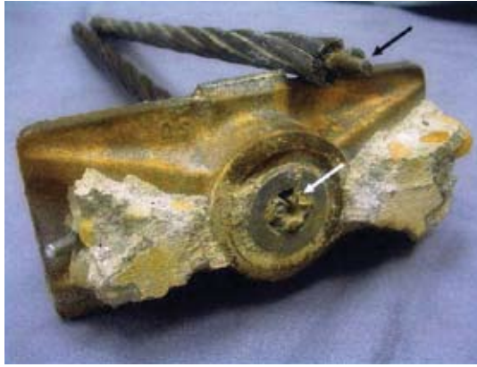
Fracture surfaces from tendon and anchor samples sent for tensile and forensic testing
