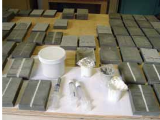
Replicas of existing shotcrete and selected repair systems at the project's architectural conservator's laboratory
