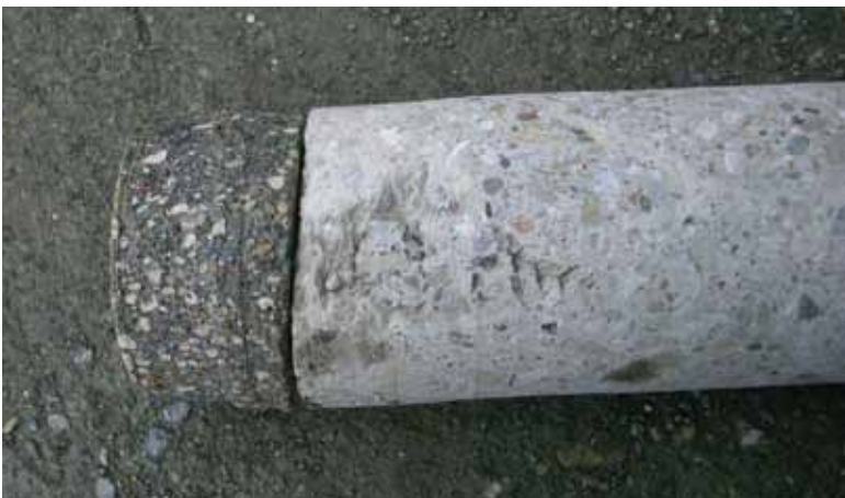
Fig. 6: Core showing the debonding of the grout at the interface of the CMU and grout
